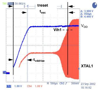
Figure 1.  $t_{osc}$  and  $t_{vddrise}$  are the Two Parameters to Evaluate, Depending on the Application
