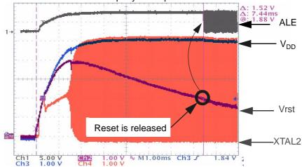
Figure 2. Reset Conditions to Properly Startup a Microcontroller
